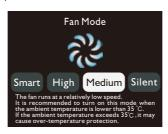
When overheat symbol appears on the light control interface, please follow the text underneath to adjust the Fan Mode to Smart or High. If the internal temperature of the lamp reaches the threshold that needs to be cooled, the lamp will automatically shut down due to overheat protection.
