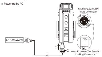
To disconnect the Neutrik® powerCon cable, pull back on the yellow release tab on the cable connector, and rotate the connector counter clockwise. Do not pull directly.
