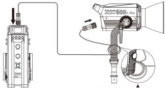
\* Hang the cable using the rope to manage and reduce tension on the cable.
